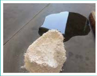
Cover spill area with AbsoPerl.
